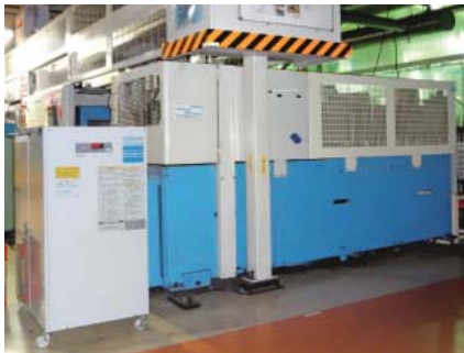
Example: Added to an Existing Immersion Chiller Built into a CNC Lathe
